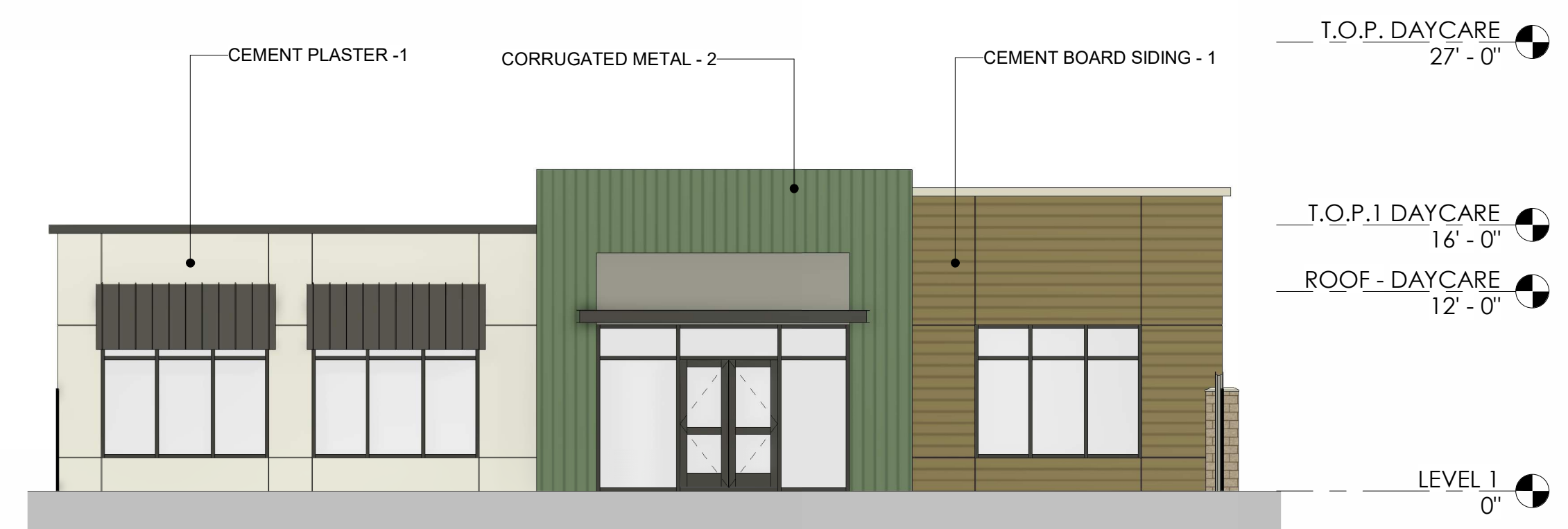
EAST ELEVATION - DAYCARE 1/8" = 1'-0" 1
